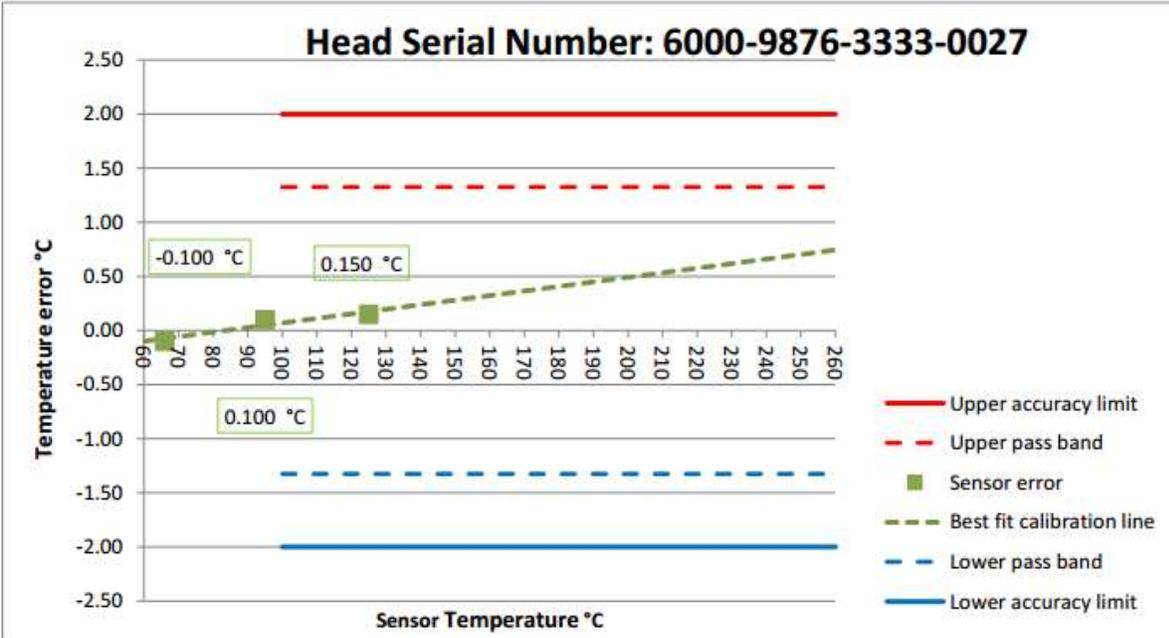
This chart has an extrapolated best-fit calibration line to illustrate that the calibration process is satisfactory for the full range of the device.
